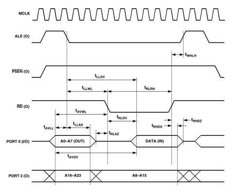
Figure 52. External Data Memory Read Cycle
